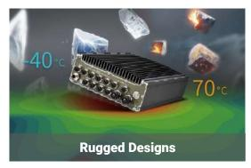
Supporting -40°C to 70°C wide-temperature operation and complies with stringent MIL-STD-810H shock and vibration standards to ensure reliable operation.
