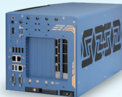
Nuvo-10208GC Series Industrial Edge AI Computer Supporting NVIDIA® GPU, Intel 14th/ 13th/ 12th Processor with Additional PCIe Slots
