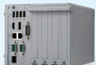
Nuvo-2822 Intel® Alder Lake N Compact Expansion Box-PC with 2x PCIe and 2x PCI Slots
