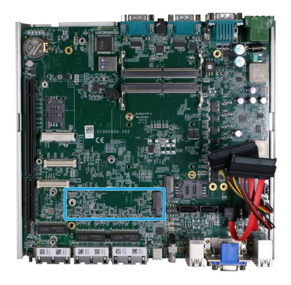
The system has a Gen4 x4 PCIe M.2 2280 slot for you to install an NVMe SSD. The M.2 NVMe SSD offers significantly better system performances when compared to a 2.5" SSD.
