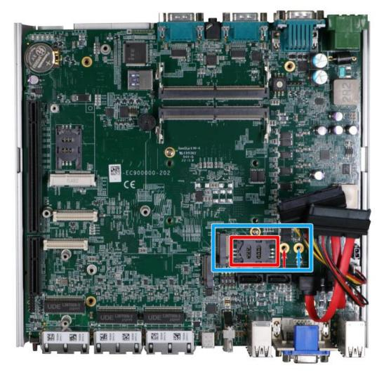
The system has an M.2 2242/ 3042/ 3052 slot (indicated in **blue rectangle**) with a 5G/ 4G SIM slot (indicated in **red rectangle**). A copper standoff is provided for you to secure onto the motherboard into the **red arrow** location for an M.2 2242/ 3042 module, or into the **blue arrow** location for an M.2 3052 module. By installing a 5G or 4G M.2 module and SIM card, you can access the internet via the provider's network.
