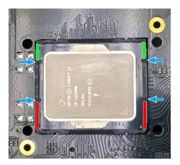
8. Make sure all thermal pad residues have been cleaned on both sides of the retention bracket. Place the CPU retention bracket (holder) on top of the CPU and hold it in place. Make sure the indicator triangle engraved on the CPU's integrated heat spreader (HIS) and the triangle indicator on the retention bracket are positioned in the same corner (indicated by blue circles).
