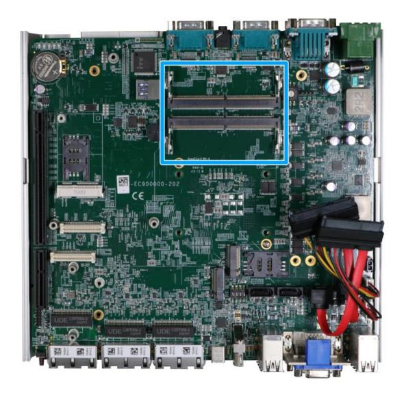
The system motherboard supports two DDR5 4800 SODIMMs memory module up to 64GB. Each slot supports single module SODIMM up to 32GB capacity.
