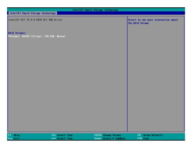
10. Press F10 to save and Esc to exit the Intel® Rapid Storage Technology configuration page.
