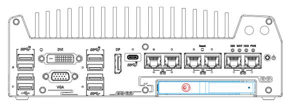
The system features a 2.5" external hot-swappable HDD/ SSD slot (indicated in blue), and secured by a lock (indicated in red). It coincides with the internal drive and can be configured into RAID 0 or 1 storage. To install HDD/ SSD into the 2.5" external hot-swappable slot, please refer to the following procedure:
