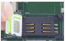
Insert Mini-SIM card with pins facing up
