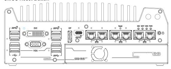
The CMOS Reset button is used to manually reset the motherboard BIOS in case of system halt or malfunction. To avoid unexpected operation, it is purposely placed behind the panel. To reset, disconnect the DC power input, and use the tip of a pen to press and hold for at least 5 seconds to reset the BIOS.
