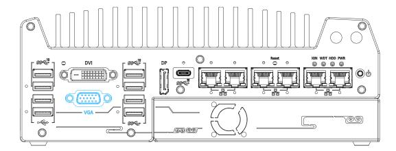
VGA connector is the most common video display connection. The VGA output supports up to 1920x1200@60Hz resolution.
