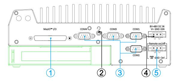
The Nuvo-9000 rear panel features MezIO<sup>TM</sup> port, four (4) COM ports, 3-pin terminal and 3-pin on/ off control. The Cassette module can be located at the bottom of the enclosure. The connectors of the installed PCI or PCIe card within the Cassette module can be accessed from this side of the panel.
