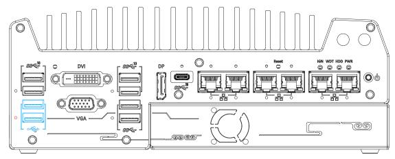
The USB2.0 ports are implemented via native xHCI (eXtensible Host Controller Interface) and are backward compatible with USB 1.1 and USB 1.0 devices. UEFI USB support is also provided so you can use USB keyboard/ mouse in UEFI shell environment. Indicated in red is a screw-lock hole for the corresponding USB port.
