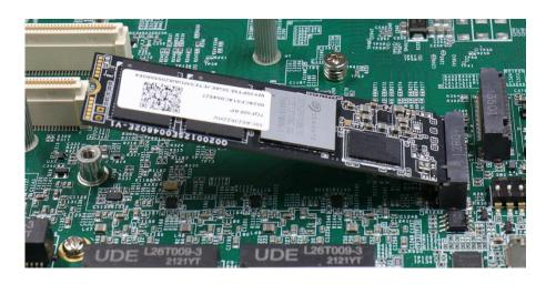
3. Gently press down and secure the module with an M2.5 P-head screw.
