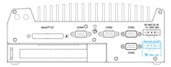
3. With DC power connected, pushing the power button will turn on the system and the PWR LED indicator will light up. Pushing the button when system is on will turn off the system. If your operating system supports ATX power mode (i.e. Microsoft Windows or Linux), pushing the power button while the system is in operation will result in a pre-defined system behavior, such as shutdown or hibernation.
