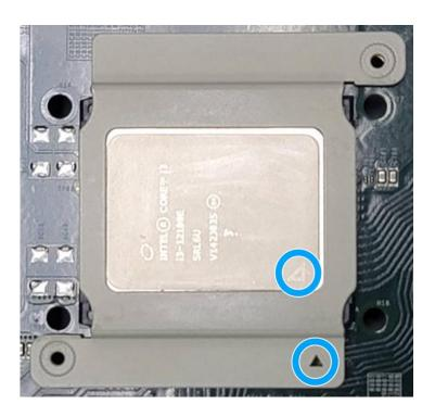
Turn the motherboard around while holding the CPU retention bracket in-place, and secure the bracket by tightening two M3 P-head screws on the other side of the motherboard.
