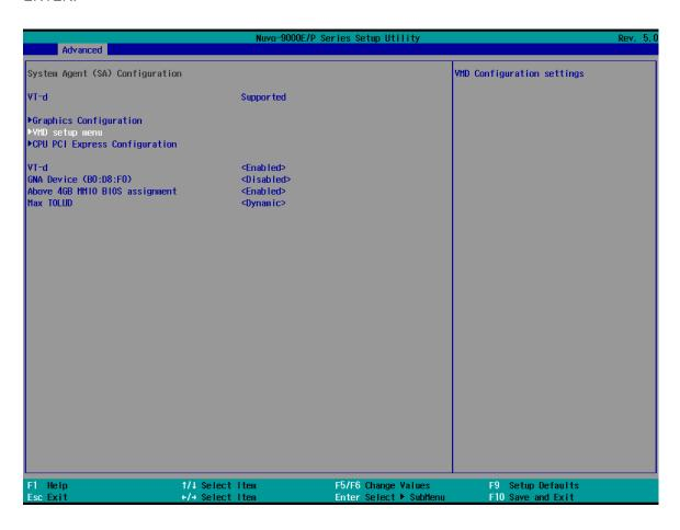
3. Select [Enable VMD controller] and press ENTER, highlight [Enabled] and press ENTER.
