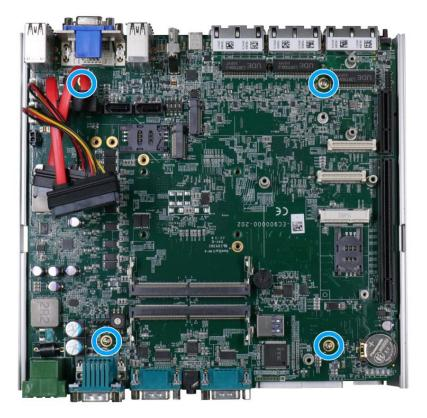
Secure motherboard with four screws
