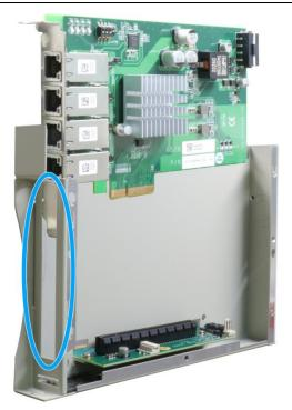
Remove bezel cover and insert the card
