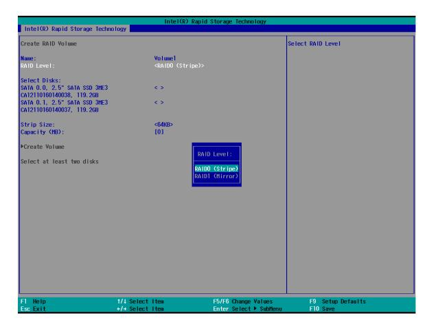
5. The Select Disks option allows you to select disk drives for your RAID volume. Highlight a drive and press ENTER, use up/ down arrow keys to highlight "x" and press ENTER to confirm the selection. A minimum of two disk drives must be selected for RAID-0 or RAID-1 configuration. Press ENTER when ready.
