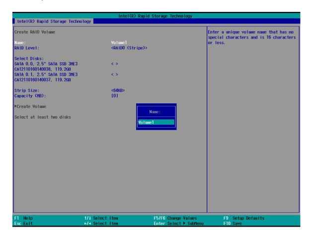
4. The RAID Level option allows you to select RAID-0 (stripping) or RAID-1 (mirror) for your RAID volume. Press ENTER when ready.
