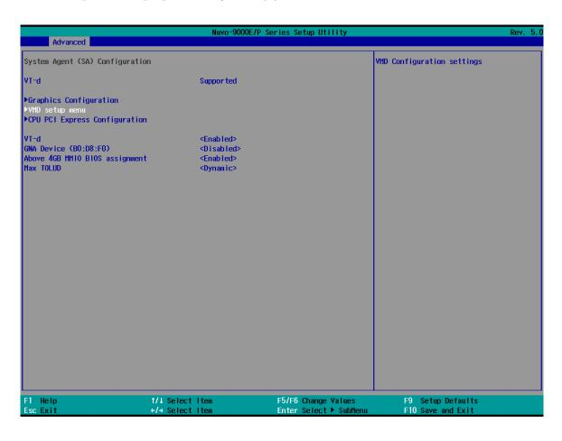
3. Highlight [Enable VMD controller], press ENTER to bring up Options, Enabled/ Disabled, select Enabled and press ENTER.
